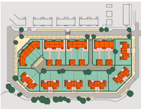
Typical Block layout incorporating semi-detached houses up to 5 bedrooms some with garages.
